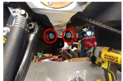
Figure 4. Centerstand Pivot Plate Left Installed
