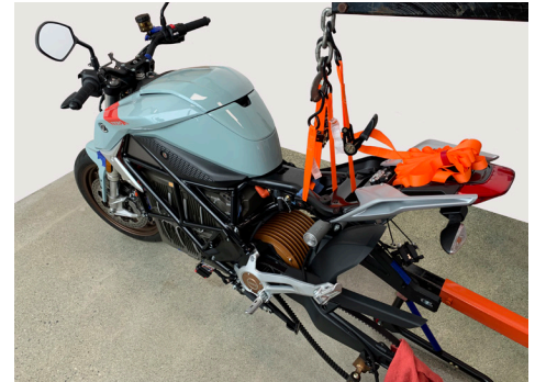
Figure 1. SR/F Lifted With Hoist From Rear
